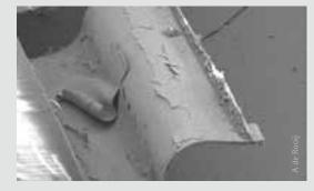
Above: Returned silver mesh solar cell interconnector - atomic oxygen corrodes silver, causing spalling of silver oxide.
