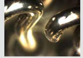
Above: Short circuiting tin whisker operation under vacuum caused whiskers to spark discharge from tip (corona discharge) and fuse, causing a plasma and current surge responsible for the failure of at least three communications satellites.
