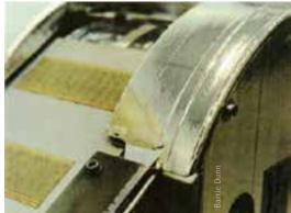
Above: Thermal cover returned from a space mission showing fringe pattern of condensed contaminant that altered its thermal properties.
